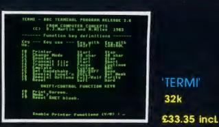
This program enables the BBC machine to act as an advanced terminal when connected to another computer or to a modem via the RS-423 (RS-232) interface. This provides facilities to transmit data from disc and the spooling of data from the 'line' to the disc or printer. Works in 3 emulation modes — normal BBC VT52 emulation or a custom mode.
